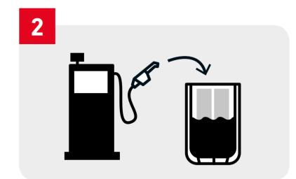
Pre-fill the filter before installing filter
