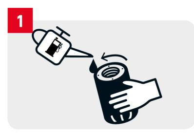
Put a bit of fuel on new gaskets for lubrication during installation
