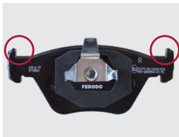
Abutment of the brake pad
