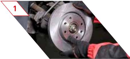
**DESCRIPTION** A deep noise with frequency below 300 Hz. It normally originates from macrovibrations of a brake system component e.g. the disc
