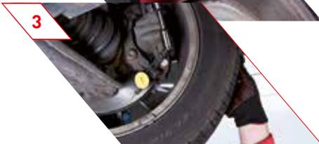
**DESCRIPTION** Noise with frequency in the range 300 - 5.000 Hz. It usually originates because of micro-vibrations in the caliper piston or in another part of the vehicle corner.
