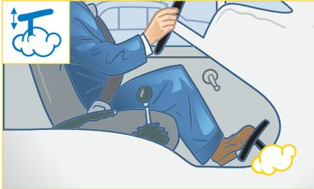
Spongy pedal feel is the experience where upon depressing the brake pedal, the brake is slow to respond, and the pedal feels spongy – softer than it should be, with excessive force required to decelerate the vehicle and excessive stroke of the pedal.
