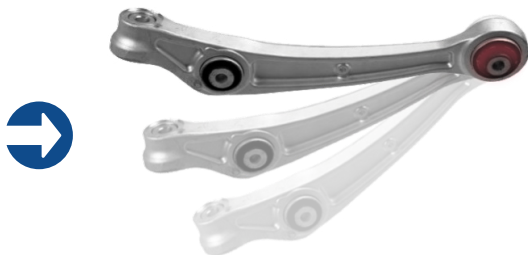
Movement of track control arm when lowering vehicle.
