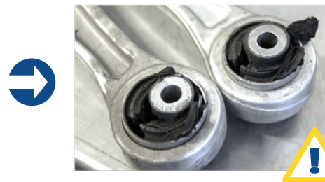
Premature wear of the track control arm bushes.
