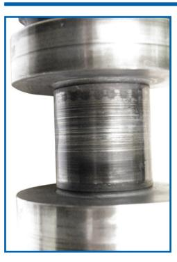
cooling failure. lubricant and replace oil and oil filter.
