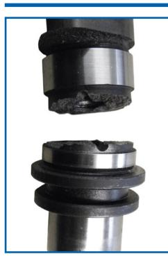
**Appearance:** Camshaft breakage between or through cam-lobes.
