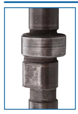
Appearance: Severe cam-lobe wear. **Causes:** Starvation or contamination of oil, tappet clearance too tight, excessive valve spring pressure. Remedy: Thoroughly flush the lubrication system, install new camshaft and followers. Adjust tappets to the correct clearances, prime with extreme pressure lubricant and replace oil and oil filter.
