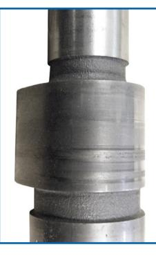
Appearance: Witness marking on base circle of cam-lobes, biased to one side. Causes: Worn hydraulic lifter and/or retainer springs. **Remedy:** Replace cam and followers if marks are deep, otherwise set tappets to correct clearance. Thoroughly flush the lubricating system and replace oil and filter.
