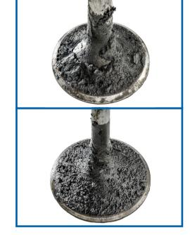
**Symptom:** Poor starting. Loss of power. Blue smoke from exhaust (when throttle closed). Cause: Excessive clearance between valve stem and guide. Valve stem seal failure or wear. Excessive oil supply due to blocked drainage paths. Incorrect grade of lubricating oil used.
