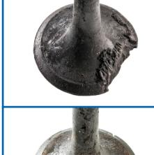
**Symptom:** Loss of power. Rough running. Cause: Valve clearance too small holding the valve off its seat. Sticking stem, poor/uneven seating or misalignment of the valve assembly. Overheating from pre-ignition. Excessive build up of carbon which flakes off the valve face to from a gas leakage path. Hard carbon particles peen into the seat surface until **Remedy:** Ensure valve clearance is to specification. of the valve assembly. Check engine timing, carburettor settings and injection timing.
