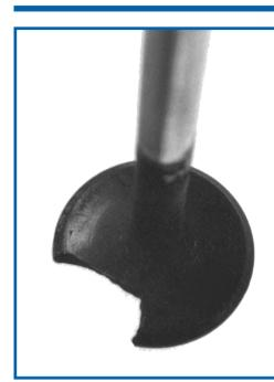
Possible seizure. Cause: Poor temperature distribution across the valve head resulting in high tensile stresses in the rim, often combined with severe deflection due to abnormal combustion pressures and temperatures. Extreme
