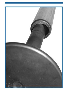
**Symptom:** Valve gear noise, high oil consumption, exhaust smoke on initial start up. Cause: Too great or too small valve stem to guide
