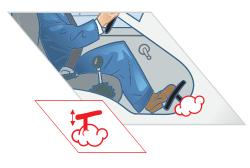
Spongy pedal feel is the experience where upon depressing the brake pedal, the brake is slow to respond, and the pedal feels spongy – softer than it should be, with excessive force required to decelerate the vehicle and excessive stroke of the pedal.
