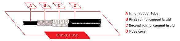
The aging process can act differently on different parts of the hose
