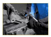
The pins must have the correct lubrication to ensure free movement and that the pin does not seize into the caliper body. Also check the condition of the slide pin rubber boots to stop water ingress.
