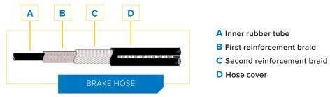
The aging process can act differently on different parts of the hose.
