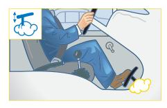
Spongy pedal feel is the experience where upon depressing the brake pedal, the brake is slow to respond, and the pedal feels spongy – softer than it should be, with excessive force required to decelerate the vehicle and excessive stroke of the pedal.
