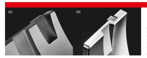
[A] The conventional locating lug is produced by punching and in some cases milling of the inner shape of the locating lug. [B] A coined locating lug is produced by means of an upsetting in one single pass. This type of a locating lug is used by most of the important OE manufacturers today.
