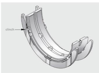
characteristics of an assembled flange bearing. for dimensions see fig. 4.
