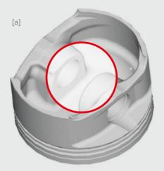
[b] The small con rod eye for this piston has a conical shape. The conical shape increases the load carrying surface of the con rod bush and the piston pin. At the same time, the rigidity of the piston is strengthened. Due to the larger load carrying surface there is less pressure on con rod bush and piston pin.
