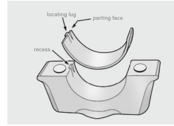
The only purpose of the locating lug of a bearing is to avoid the bearing being assembled in an incorrect position into the housing. The housing bore has a recess in which the locating lug fits. The locating lug does not prevent the bearing from turning in the housing.
