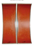
Bearing shells lined with the A-650 Al alloy substrate after endurance testing on a rig with 80 MPa for 250 h
