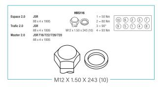
If the bolt is not turned enough an inadequate load level will be generated. However if the bolt is turned too far into yield the bolt is likely to fail.
