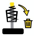
4. Remove the fixing nut and dismantle the assembly.
