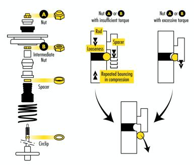
1. On vehicles equipped with cir-clip shock absorbers, it is common to see a cir-clip ring that has moved out of position and damaged the piston rod. This fault is caused by improper tightening of the nut securing the series of upper elements against the cir-clip. (See nut "B" in drawing.)
