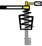
9. Once the spring is compressed and secured, **use the correct tooling** (hollow spanner, ratchet and socket combination) **to remove the nut on top of the strut rod**.
