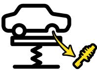
7. Carefully extract the strut assembly from the vehicle. In some vehicle models, it will be necessary to compress the spring prior to extracting the strut assembly.
