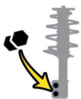
4. Attach the completed strut assembly onto the steering knuckle. Leave the bolts only finger-tight, allowing the assembly to move freely.
