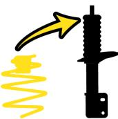
1. Install the spring in its correct position on the strut's spring seat
