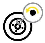
2. Before lifting the vehicle, loosen (but do not remove) bolts securing the wheel
