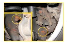
A fatigue failure of a ball pin neck can cause a driver to lose control of the vehicle. The combination of an induction hardened ball pin neck and MOOG's patented carbon fibre bearing not only enhances both the performance and the service life of the ball joint but also improves driver safety.
