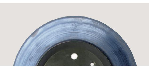
• If necessary, replace both discs on the axle.
