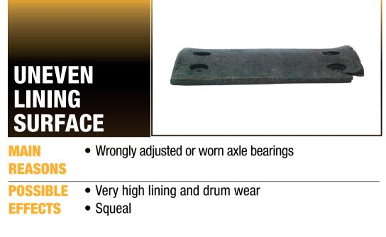
SOLUTION Replace linings, replace wheel bearing and replace or grind drum as appropriate
