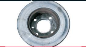
What caused it? Excessive hub run-out and uneven disc-to-pad contact generates vibration that causes localized heat.
