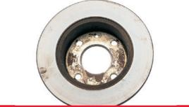
What caused it? Contamination on hub surface. This results in misalignment during mounting leading to irregular contact between pad and disc surfaces and irregular wear of the disc.
