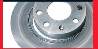
What caused it? Mechanical stress caused by misalignment and wrong assembly/positioning of the caliper and the disc. This causes asymmetrical wear of the braking surface.
