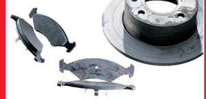
What caused it? One brake pad is in constant contact with disc This causes the pad to wear down to the metal backplate
