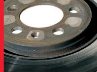
What caused it? Incorrect assembly of the caliper and/or pads can cause the pads being at a different angle to the disc, each side wearing at changed rates. Blue spots are generated by severe localized overheating. What is the effect? Progressive onset of vibrations, due to heat spots. Probable reducing of the brake efficiency. How do you fix it? Inspect and repair caliper. Replace pads.
