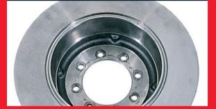
What caused it? Tightening sequence incorrect, not enough tightening torque used. What is the effect? Vibration on initial brake applications
