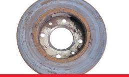
What caused it? Friction material deposits on disc surface. This usually appears where bad quality brake pads have been installed.
