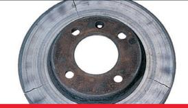
What caused it? Blue spots are a result of rising cracks caused by metallurgical change in the surface material making it hard and brittle. This is common in cases of overloading the brakes beyond normal design limits. This could result from aggressive driving, excessive payload or intensive/unusual brake use. What is the effect? Reducing brake performance,
