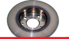
What caused it? Poor bedding-in. If not accurately bedded, surfaces where friction appears get overheated. This leads to a metallurgical change on the friction surface.
