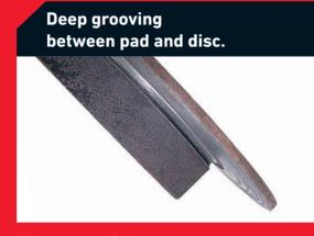
What caused it? Extreme pad and disc wear may result in movement of the backplate within caliper. In this case, the backplate of the worn pad has separated from its seat within caliper causing grooving between hat and disc surface.
