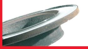
What caused it? Discs were not inspected regularly or replaced at the correct moment. What is the effect? Lower performance, excessive noise and vibration while braking How do you fix it? Fully inspect the braking system and associated components. Replace any failed components and fit new discs with the right torque and sequence recommended by the manufacturer during tightening.
