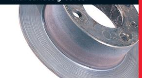
What caused it? Excessive or full brake pad wear results the brake pad backplate contacting the disc (metal to metal). This will make grooves in the disc surface.
