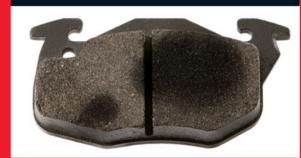
**Appearance.** Contamination of the Friction material with either oil, grease or brake fluid.
