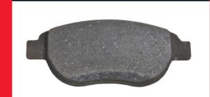
Appearance. Unequal wear on the pad surface. What caused it? An unevenly worn brake disc or 'wear lip' on the disc will cause this pattern of wear on the brake pad.
