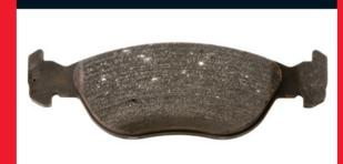
**Appearance.** Metal ingrained on the friction surface.
