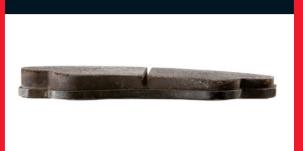
**Appearance.** Irregular wear or tapered pads What caused it? Distortion of the caliper and the slides are sticking and needless caliper clearance.
