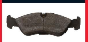
Appearance. Small cracks in the middle of the pad What caused it? Cracks illustrate that the caliper is sticking. The piston flexes the back plate causing the back plate to bend, cracking the friction material.
