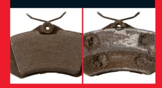
Appearance. Rust between the friction material and back plate.
