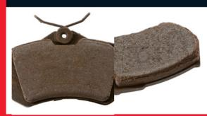
**Appearance.** Unequal wear pattern on the pad. What caused it? Brake pad is sticking within the caliper. This causes the brake pad to stay in contact with the disc with associated needless pad temperature.
