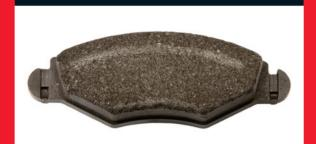
Appearance. Unequal wear pattern on the pad What caused it? No full contact between brake pad and disc, disc scoring by dust or excessive wear. New pads with a worn disc may also show
