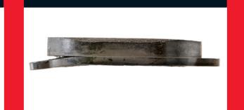
Appearance. A back plate that is damaged. What caused it? Not correctly assembled, or needless force used during fitting.
