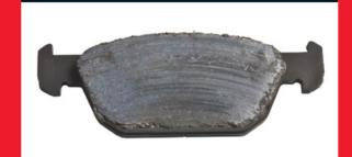
Appearance. The brake pad friction material is glazed
