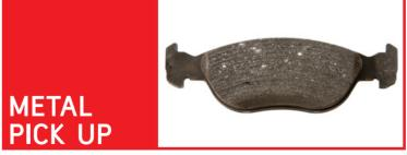
**APPEARANCE** Metal pick-up (or ingrained metal) on the friction surface
