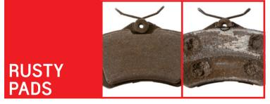
**APPEARANCE** Rust between the friction material and back plate
