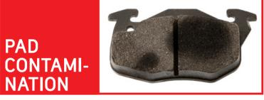
**APPEARANCE** Friction material is contaminated with either oil, grease or brake fluid
