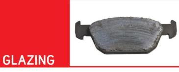
**APPEARANCE** The brake pad friction material is glazed **CAUSE** • High intermittent pad temperature over short time periods • Overly harsh braking during the bedding-in period **EFFECT** Temporary reductions in brake performance **REMEDY** • If light glazing is evident, no action is required
