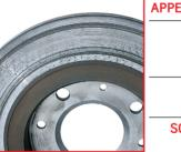
**APPEARANCE** Grooving on the disc **CAUSE** The deep grooves are caused by loose abrasive particles between the pads and disc. Foreign debris may enter from outside the brake system (road, dirt, water) or from poorly mixed friction material **EFFECT** Noise during braking and normal running, and lower brake efficiency due to reduced braking contact surface **SOLUTION** Replace pads and discs
