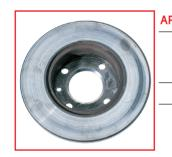
APPEARANCE Blue spots, darker colour of some disc areas. Evidence of localised overheating CAUSE Excessive hub run-out. Uneven disc-to-pad contact generates excessive oscillation which in turn leads to localised heat generation - subsequently discolouration (blueing)
