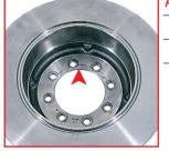
CAUSE Tightening sequence incorrect. Insufficient tightening torque used
