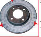
**CAUSE** The blue spots are symptomatic of rising cracks. These are caused by metallurgical change in the surface material making it hard and brittle. This is typical of overloading the brakes beyond normal design limits. This could result from intensive or unusual brake use e.g. aggressive driving or excessive payload EFFECT Brake fade/reduced brake performance, noise, vibrations
