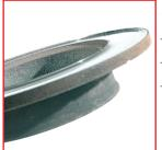
APPEARANCE Excessive wear. Disc thickness is lower than manufacturer's recommended 'Minimum Thickness' **CAUSE** Discs were not checked regularly or changed at the correct point EFFECT Performance decrease, vibration and excessive noise while braking SOLUTION Full inspection of braking system and associated components. Replace any failed components and fit new discs observing manufacturer's recommended torque and sequence during tightening. Ensure future checking and periodic maintenance
