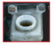
**PPEARANCE** Abnormal brake pedal behaviour Brown contaminated brake fluid
