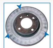
**APPEARANCE** Radial fractures/blue spots corresponding to the venting frames CAUSE The blue spots are symptomatic of rising cracks. These are caused by metallurgical change in the surface material making it hard and brittle. This is typical of overloading the brakes beyond normal design limits. This could result from intensive or unusual brake use e.g. aggressive driving or excessive payload
