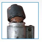
**APPEARANCE** Rust around brake cylinder pins CAUSE Limited usage of brakes, improper lubrication during assembly **EFFECT** No brake force, vehicle tends to pull to one side during braking **REMEDY** Replace or overhaul brake cylinder
