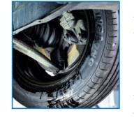
**APPEARANCE** Wet spots at brake drum **CAUSE** Brake cylinder leakage **EFFECT** Mushy brake pedal, brake pedal sinks to the floor, limited brake performance. Due to brake fluid on the brake lining the vehicle may tend to pull to one side during braking **REMEDY** Replace brake cylinder
