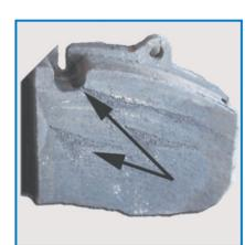
**APPEARANCE** Excessively worn out discs and pads
