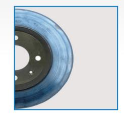
**APPEARANCE** Blue stripes on the disc indicating a physical change due to overheating
