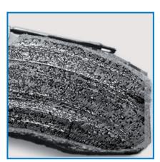
**APPEARANCE** Contaminated pad friction material
