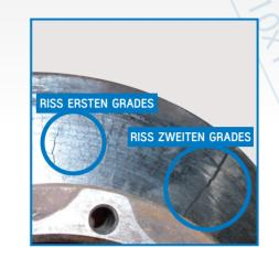
**APPEARANCE** Disc surface features 1st and 2nd degree crack
