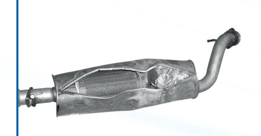
Silencer housing has exploded due to condensation of unburned fuel (HC) inside the silencer.
