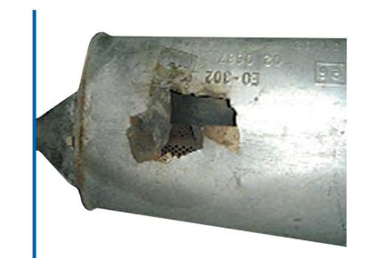
Perforated exhaust housing. This failure is common in mono-layer silencers due to the accumulation of water inside.
