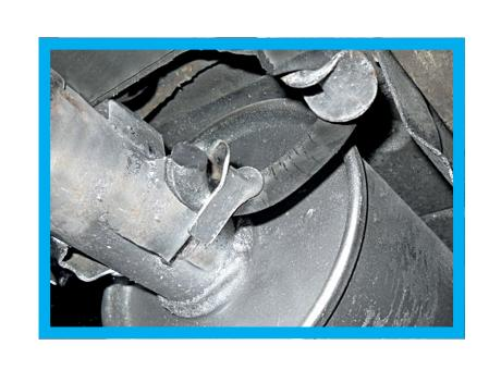
Worn-out or broken rubber hangers produce a perfectly round cut, around the welded joint where the pipe connects to the silencer housing. This is a common failure where the silencer has been replaced using the old rubber hangers.
