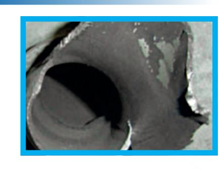
Worn-out or broken engine mountings or flexible drive shaft joints produce a typical irregularly shaped fracture which destroys the pipe a few centimetres behind the connection to the silencer.
