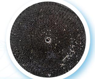
Chemical pollution of the monolith due to the use of lead, generally coming from leaded gasoline or anti-detonant additives not designed for use in catalysed vehicles.
