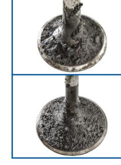
**Symptom:** Poor starting. Loss of power. Blue smoke from exhaust (when throttle closed).
