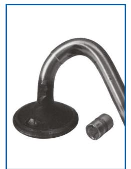
**Symptom:** Excessive mechanical noise, bent stem and possible head detachment.
