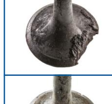
**Symptom:** Loss of power. Rough running. Cause: Valve clearance too small holding the valve off its seat. Sticking stem, poor/uneven seating or misalignment of the valve assembly. Overheating from pre-ignition. Excessive build up of carbon which flakes off the valve face to from a gas leakage path. Hard carbon particles peen into the seat surface until
