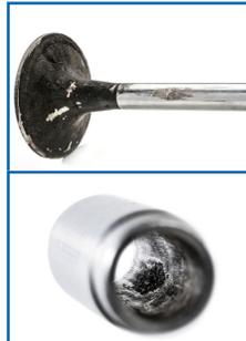
**Symptom:** Poor performance due to low compression. Mechanical breakage due to sticking valves.
