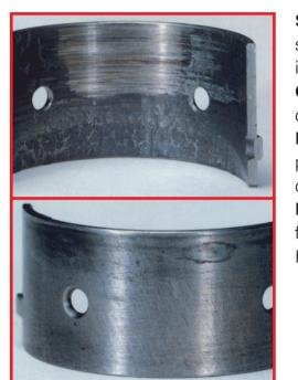
**Symptom:** Localised surface disruption of bearing surface. The back of the bearing will be marked or indented behind the area of damage. **Cause:** Foreign material assembled between the back
