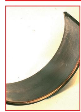
Symptom: Inner surface of bearing contacts journal fillet on one or both ends of the shell. Lining material is worn down at bearing edge(s) along its circumference.
