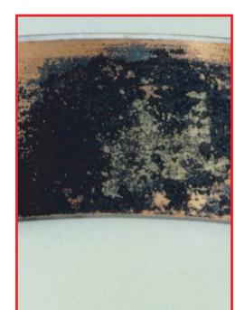
**Symptom:** Corrosion of the bearing material. The surface will be worn and discoloured with a porous appearance.
