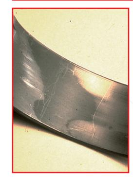
**Symptom:** Overplate wear only in the crown area of bearing shell towards the edge zones. Worn zones are shifted against each other in circumferential direction. **Cause:** Centerlines of bearing and journal are not
