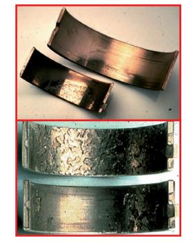
**Symptom:** Breakouts of lining material showing "barkbeetle" pattern in main loaded zone of bearing. **Cause:** Overloaded bearing material due to: Installation of non suitable bearings. Edge loading of bearing due to sheft deformation or imperfect sheft geometry. Irregular combustion. Engine tuning.
