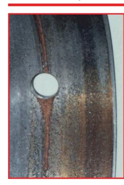
**Symptom:** Premature bearing wear. The internal surfaces may appear scratched and/or have embedded debris. Erosion may also be visible adjacent to an oil groove or hole.
