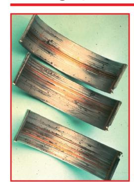
**Symptom:** Isolated deep scores in lining surface. **Cause:** Isolated debris particles from casting or grinding processes passed the bearing without being embedded. Blocked oil filter.
