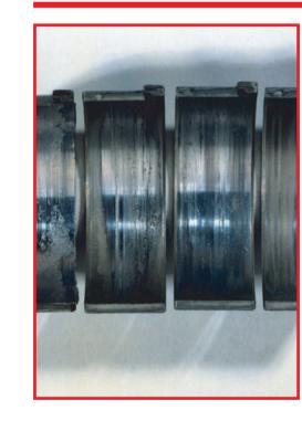
**Symptom:** Wiping or melting of the bearing surface which may progress to fatigue and destruction of the
