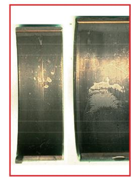
**Symptom:** Overplate material is locally resolved from sliding surface. Faulty spots are located symmetric or centric in bearing sliding surface or behind end of an oilgroove.
