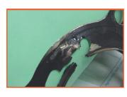
Damage: A cylinder head gasket is a delicate component and easily damaged. Always inspect a gasket before assembly and never install one that has been folded or creased. Never re-use a cylinder head gasket.
