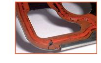
Distortion: Cylinder head gaskets are designed to seal flat surfaces. Distorted cylinder heads and engine blocks will impair gasket sealing performance.
