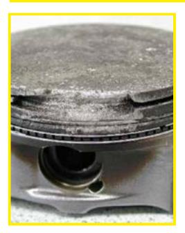
**Cause:** Overexpansion of ring when fitting the piston. Faulty fitting of piston or ring into engine block. Excessive pressure or worn piston grooves. **Remedy:** Replace defective parts. Ensure piston and rings are correctly fitted. Use piston ring expander to prevent overstressing of ring during assembly. Check if the piston grooves are to specification.
