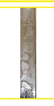
**Cause:** Overheating due to insufficient oil or coolant supply.
