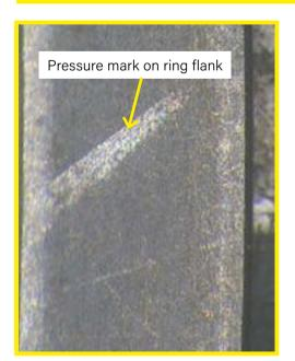
**Cause:** Dirt or debris in engine. Secondary damage due to overheating and seized piston(s). Remedy: Replace defective parts, clean engine, change oil, oil filter and air filter.
