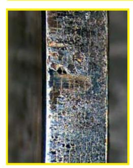
Cause: Insufficient lubrication, overheating due to high frictional loads.
