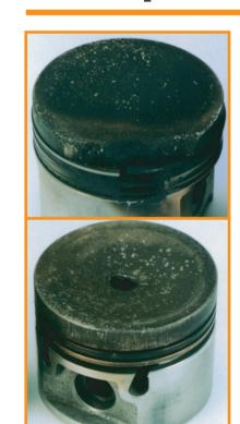
**Symptom:** Engine noise: Pinging/loss of power. **Cause:** Heat range of spark plugs too low. Mixture too lean.
