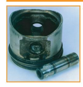
**Symptom:** Engine noise. **Cause:** Lack of clearance between rod bushing and pin. Lack of lubrication between piston pin and pin bore during installation.
