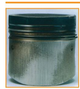
**Symptom:** Oil consumption. **Cause:** Bent connecting rod or misaligned small end bush. Excessive crankshaft end float. Liners not installed
