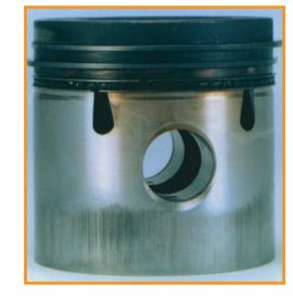
**Symptom:** Engine does not develop normal full power. Engine may overheat. **Cause:** Insufficient piston skirt to cylinder running
