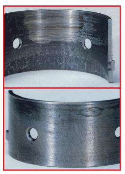
**Symptom:** Localised surface disruption of bearing surface. The back of the bearing will be marked or ndented behind the area of damage. **Cause:** Foreign material assembled between the back
