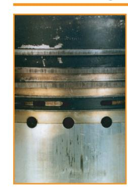
**Symptom:** Oil consumption, with possible fumes from engine breather. **Cause:** Excessive cylinder surface temperature. Margin
