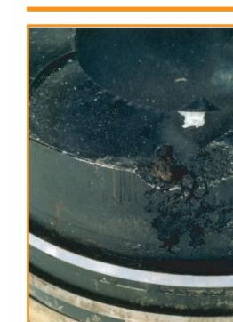
Symptom: Loss of power, emission of fumes from engine breather. Exhaust smoke.
