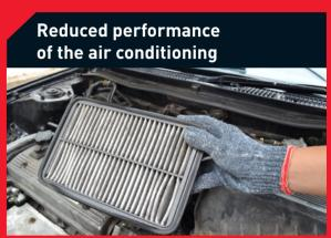
Possible cause: Cabin filter is clogged with dirt and dust and reduces the air flow Solution: Replace the cabin filter
