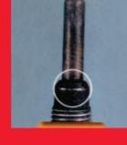
• Tightening torque too high. • Inappropriate tool used or damage of the cylinder head hole thread.
