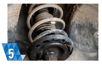
**EXCESSIVE VIBRATION (All Sensors)** Road vibrations, worn suspension parts or improper tightening torque loosen or damage sensors.
