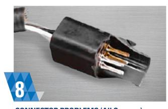
**CONNECTOR PROBLEMS (All Sensors)** Corroded or loose connectors causing poor electrical connections.
