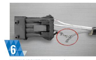
**WIRING ISSUES (All Sensors)** Broken, frayed or shorted wiring or connectors leading to or from the sensor.
