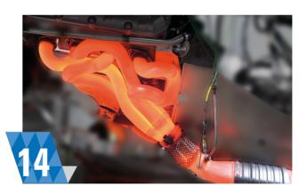
**MECHANICAL HEAT DAMAGE** (for DPS, EGT, lambda and NOx): Prolonged exposure to extreme heat can cause sensor degradation. Repeated thermal cycling (Heating and cooling) can lead to cracks or breakages in sensor internal components.
