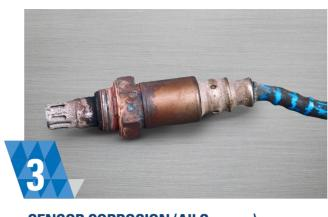
**SENSOR CORROSION (All Sensors)** Moisture and salt corrode the sensor connectors.
