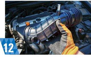
**VACUM LEAKS (For MAF)** Leaks in the intake system can introduce unmetered air, causing inaccurate MAF sensor readings.
