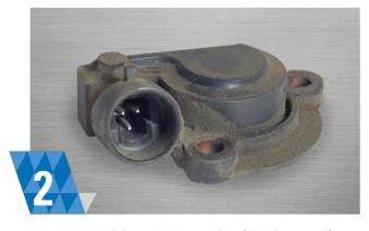
**DIRT AND CONTAMINATION (All Sensors)** Dust, dirt, and oil can accumulate on the sensor, affecting its ability to operate accurately.
