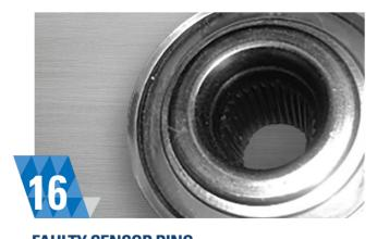
**FAULTY SENSOR RING** (for CMP, CKP and WSS) Cracked or worn sensor rings provide inaccurate data.
