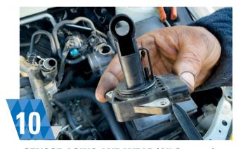
**SENSOR AGING AND WEAR (All Sensors)** Over time, sensors can wear out due to normal aging. The sensor internal components can become less responsive, leading to slower reaction time or inadequate readings.
