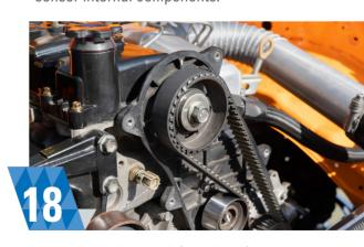
TIMING PROBLEMS (For CMP) Worn or improperly aligned timing belts or chains affecting the camshaft position.
