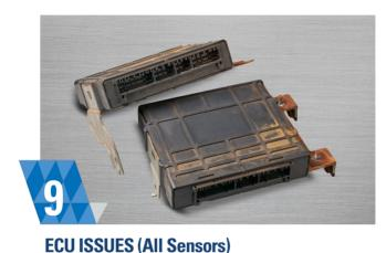
In rare cases, electronic control unit (ECU) may be faulty and not correctly interpreting the sensor signals.
