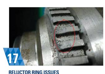
(for CMP, CKP and WSS inductor sensors) Damage, misalignment or excessive dirt on the reluctor ring (Toothed wheel that the sensor reads) can cause improper readings.
