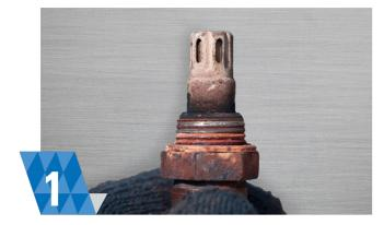
**FAULTY SENSOR (All Sensors)** The sensor itself, due to a manufacturing or transportation issue, may be defective.
