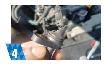
**MECHANICAL DAMAGE (All Sensors)** Physical damage to the sensor due to improper handling or impact.
