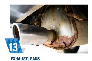
(For DPS, EGT, lambda and NOx) Leaks in the exhaust system (before and after DPF or catalytic converter) or intake can result in abnormal sensor readings.
